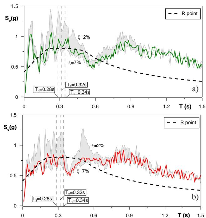
Figure 5. The response acceleration spectrum to the AQG main shock ( $\xi=5\%$ ) compared with the elastic spectrum relative to the target PGA (R point in Figure 3): (a) N-S component, (b) E-W component. The dashed gray-lines represent the three principal modal period of the substructure A3.
