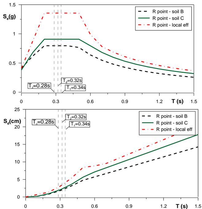
Figure 7. Comparison between the AQG average spectrum, the Roio spectrum and the hypothesized spectrum due to the local effects. The dashed gray-lines represent the three principal modal period of the substructure A3.
