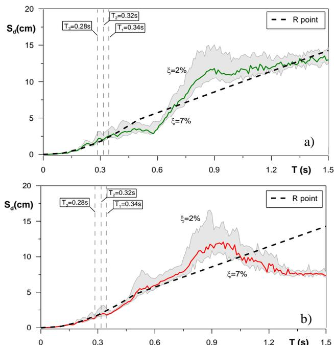
Figure 6. The response displacement spectrum to the AQG main shock ( $\xi=5\%$ ) compared with the elastic spectrum relative to the target PGA (R point in Figure 3): (a) N-S component, (b) E-W component. The dashed gray-lines represent the three principal modal period of the substructure A3.
